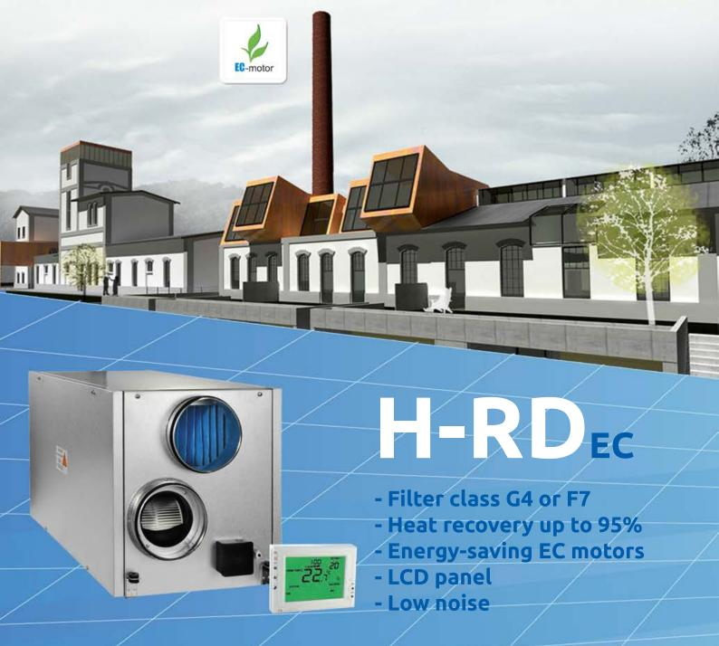
Compact energy efficient air handling unit designed for comfort ventilation of houses and flats. The unit is equipped with filtered air inlet and outlet, a country-flow heat exchanger with efficiency up to 95 %, two centrifugal fans and electric or water heater and fans with EC-motors. EC-motors reduce energy consumption and ensure high efficiency and low noise levels at the same time. The unit can be fully controlled.
